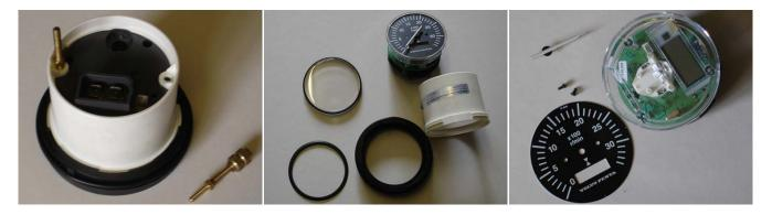
The old LCD display can be prised out with a blade under the edge - the ribbon cable 'can' be pulled out but it is better to try and lever up the sides of the white terminal block to release (5,6,7):
