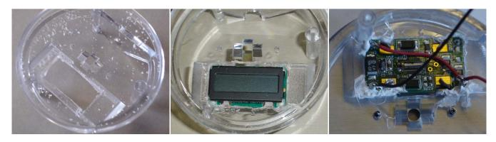
The parts of the tacho separated to solder on the wires to the input terminals (12) on the back of the circuit board then re-assembled (13) Finished meter (14)
